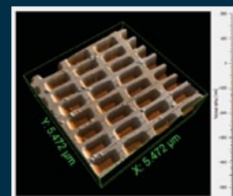
Measurement of critical dimensions in silicon oxide features
