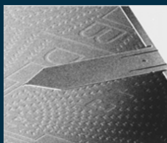
AFM SmartActiveProbe in SEM
